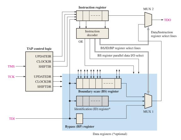
FIGURE 10-46 Boundary scan logic diagram.
