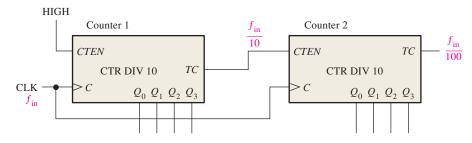
FIGURE 9-37 A modulus-100 counter using two cascaded decade counters.
