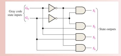
FIGURE 6-66 State decoder logic.
