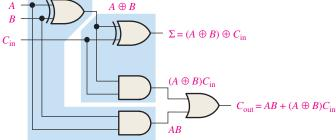
(a) Logic required to form the sum of three bits
