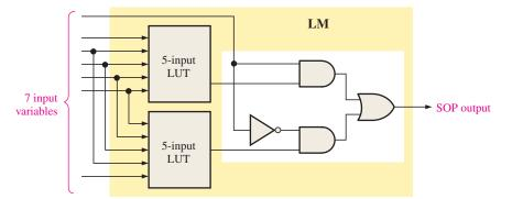
**FIGURE 10–29** Expansion of a logic module (LM) to produce a 7-variable SOP function in the extended LUT mode.
