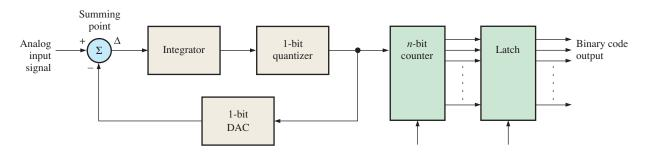
FIGURE 12-22 One type of sigma-delta ADC.
