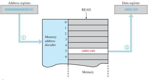
(1) Address  $5_{10}$  is placed on address bus and followed by the read signal.
