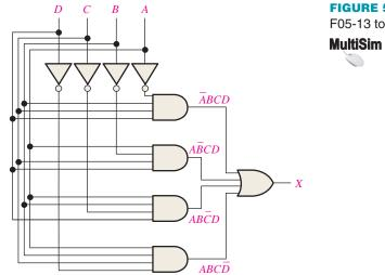
FIGURE 5-13 Open file F05-13 to verify the operation. MultiSim
