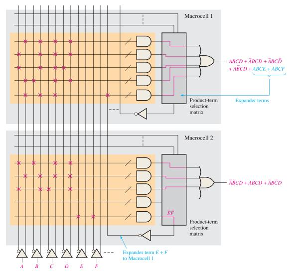
**FIGURE 10–12** Simplified illustration of using a shared expander term from another macrocell to increase an SOP expression. The red Xs and lines represent the connections produced in the hardware by the software compiler running the programmed design.
