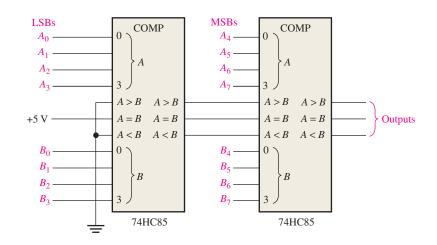
FIGURE 6–25 An 8-bit magnitude comparator using two 74HC85s.
