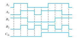
**9.** The following sequences of bits (right-most bit first) appear on the inputs to a 4-bit parallel adder. Determine the resulting sequence of bits on each sum output.
