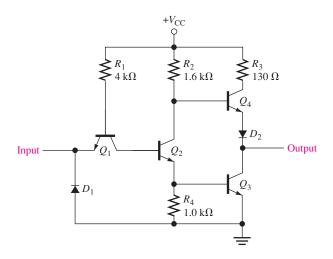
FIGURE 15–27 A standard TTL inverter circuit.
