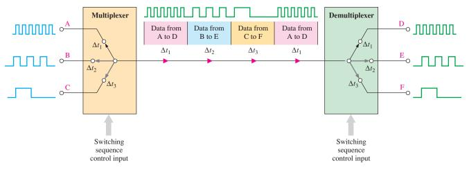
FIGURE 1-24 Illustration of a basic multiplexing/demultiplexing application.
