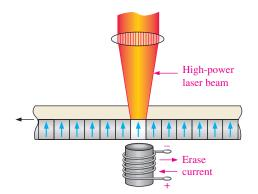
(d) Erasing: The electromagnetic field is reversed as the highpower laser beam heats the spot, causing the magnetic particles to be restored to the original polarity.
