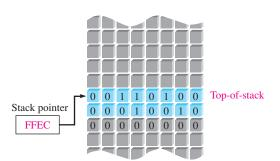
(b) The stack pointer is decremented by two and the data word 0001001000110100 is placed in the two locations prior to the original stack pointer location.
