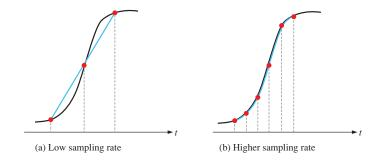
**FIGURE 1–49** Example of sampling a waveform. The dashed lines represent the clock (sampling) rate. The incoming signal is black and the resulting representation is blue. The red dots are the points at which the waveform values are sampled.
