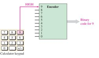
**FIGURE 1–22** An encoder used to encode a calculator keystroke into a binary code for storage or for calculation.
