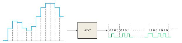
**FIGURE 12-6** Basic function of an analog-to-digital converter (ADC) (The binary codes and number of bits are arbitrarily chosen for illustration only). The ADC output waveform that represents the binary codes is also shown.
