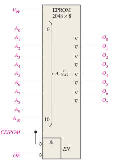
**FIGURE 11–31** The logic symbol for a 2048  $\times$  8 EPROM.
