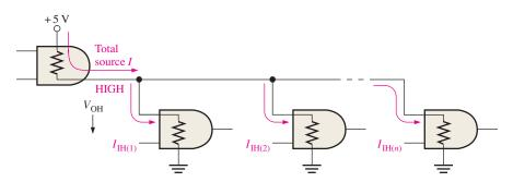
FIGURE 15–13 HIGH-state TTL loading.
