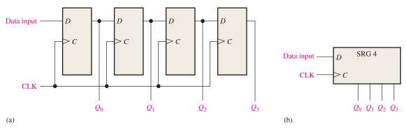
**FIGURE 8–6** A serial in/parallel out shift register.
