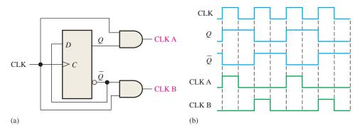
**FIGURE 7–61** Two-phase clock generator with ideal waveforms. Open file F07-61 and verify the operation.
