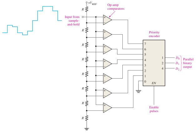
FIGURE 12–12 A 3-bit flash ADC.
