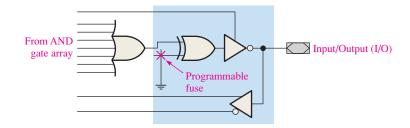
(c) Programmable polarity output
