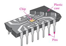
**FIGURE 1–38** Cutaway view of one type of fixed-function IC package (dual in-line package) showing the chip mounted inside, with connections to input and output pins.
