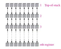
FIGURE 11-52 Register stack.
