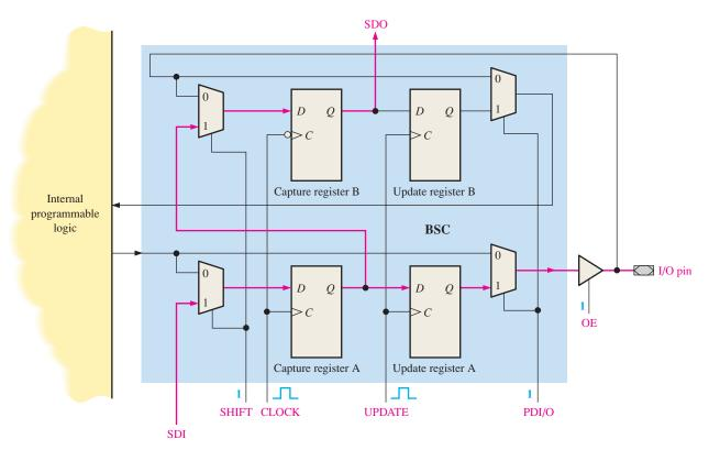
**FIGURE 10–53** Data path for transferring data from the SDI to a device output pin and the SDO. There is a 1 on the SHIFT line, a 1 on the PDI/O line and a 1 on the OE line. A pulse is applied to the CLOCK line followed by a pulse on the UPDATE line.
