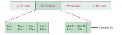
FIGURE 13-47 T1 channel transmission.
