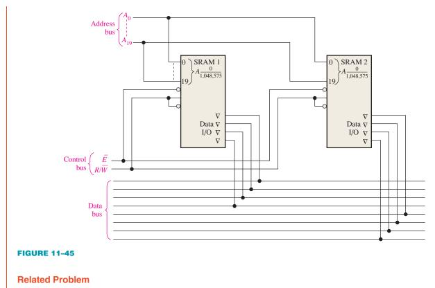
Use  $1M \times 8$  SRAMs to create a  $1M \times 16$  SRAM.
