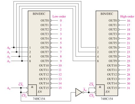
FIGURE 6-30 A 5-bit decoder using 74HC154s.
