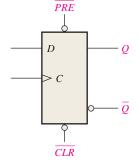
**FIGURE 7-25** Logic symbol for a D flip-flop with active-LOW preset and clear inputs.
