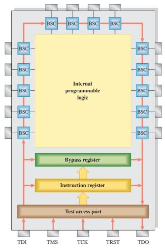
**FIGURE 10–45** Greatly simplified diagram of a JTAG compliant (IEEE Std. 1149.1) programmable logic device (CPLD or FPGA). The BSCs (boundary scan cells) form the boundary scan register. Only a small number of BSCs are shown for illustration.
