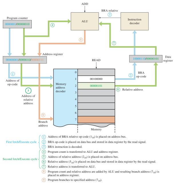
FIGURE 14–21 Illustration of relative addressing (branching).
