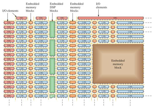
FIGURE 10-33 Example FPGA block diagram.
