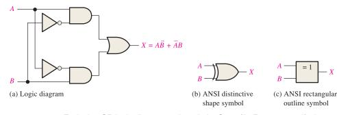
**FIGURE 5-5** Exclusive-OR logic diagram and symbols. Open file F05-05 to verify the operation.
