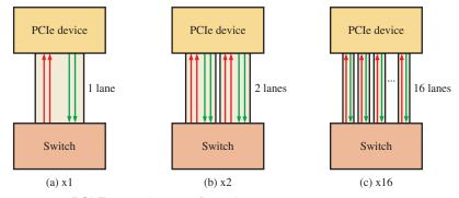
FIGURE 13–57 PCI-Express lane configurations.
