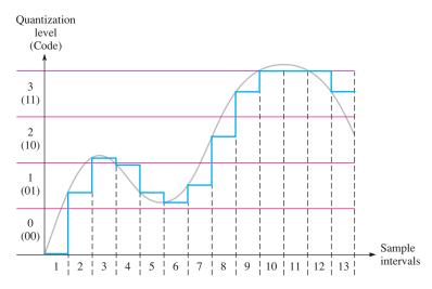
**FIGURE 12–7** Sample-and-hold output waveform with four quantization levels. The original analog waveform is shown in light gray for reference.
