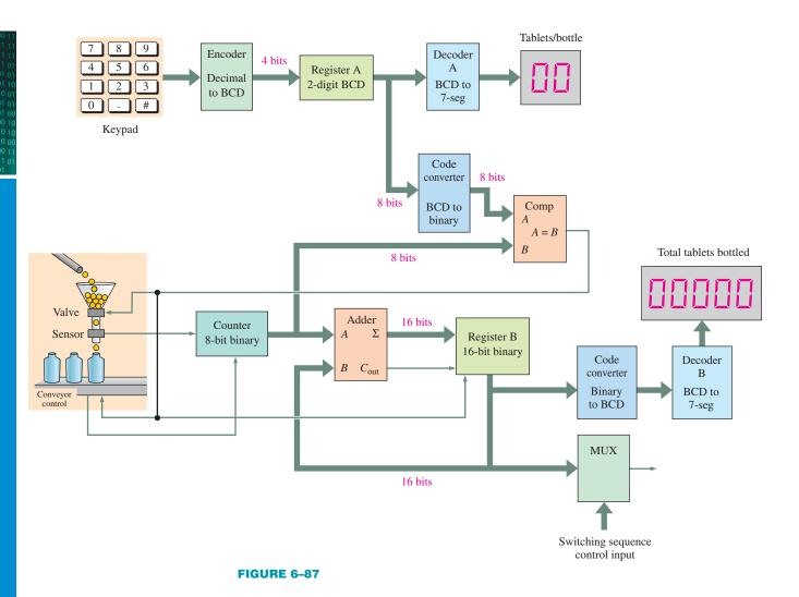
the adder goes back into Register B. Use 74HC283s to implement this function and draw a complete logic diagram including pin numbers. This is similar to the system in Section 1–4.
