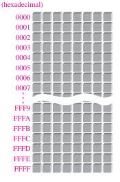
FIGURE 11–55 Representation of a 64 kB memory with the 16-bit addresses expressed in hexadecimal.
