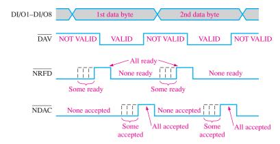
FIGURE 13-59 Timing diagram for the GPIB handshaking sequence.
