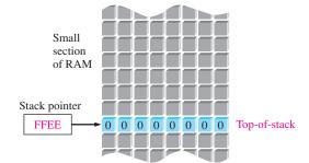
(a) The stack pointer is initially at FFEE before the data word 0001001000110100 (1234) is pushed onto the stack.
