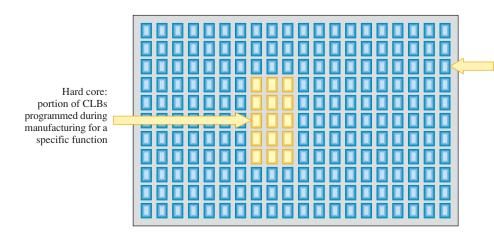
**FIGURE 10–32** Basic idea of a hard-core function embedded in an FPGA.
