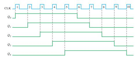
FIGURE 8–23 Timing sequence for a 5-bit Johnson counter.
