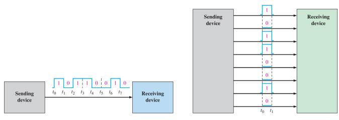
(a) Serial transfer of 8 bits of binary data. Interval  $t_0$  to  $t_1$  is first.
