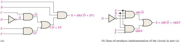
**FIGURE 5–10** Logic circuits for  $X = AB(C\overline{D} + EF) = ABC\overline{D} + ABEF$ .
