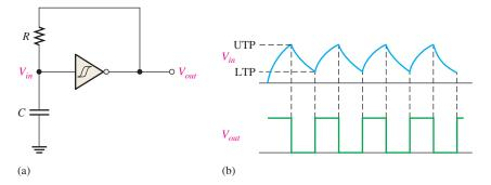
FIGURE 7-55 Basic astable multivibrator using a Schmitt trigger.
