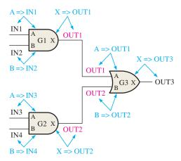
**FIGURE 5–40** Illustration of the instantiation statements and port mapping applied to the AND-OR logic. Signals are shown in red.
