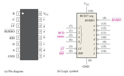
FIGURE 6-34 The 74HC47 BCD-to-7-segment decoder/driver.
