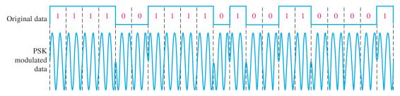
FIGURE 13-22 Illustration of phase-shift keying (PSK).
