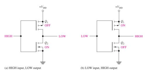
FIGURE 15–18 Operation of a CMOS inverter.
