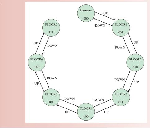
FIGURE 9–63 Floor counter state diagram.
