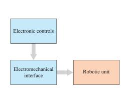
(a) Mechatronic system block diagram
