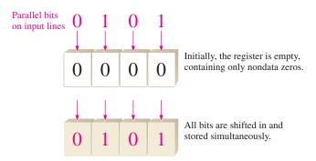
FIGURE 1-26 Example of the operation of a 4-bit parallel shift register.
