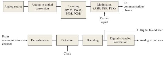
FIGURE 13–39 General function block diagram of a data transmission system.
