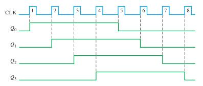
FIGURE 8-22 Timing sequence for a 4-bit Johnson counter.
