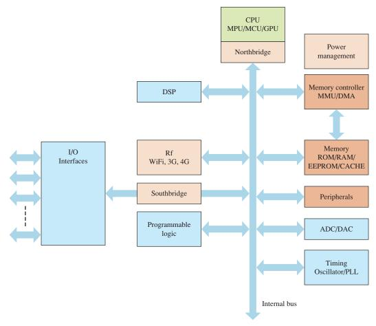
FIGURE 14–38 Generic block diagram of a typical SoC.
