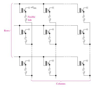
**FIGURE 11–30** MOS PROM array with fusible links. (All drains are commonly connected to  $V_{\text{DD}}$ .)
