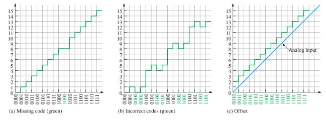
FIGURE 12-24 Illustrations of analog-to-digital conversion errors.
