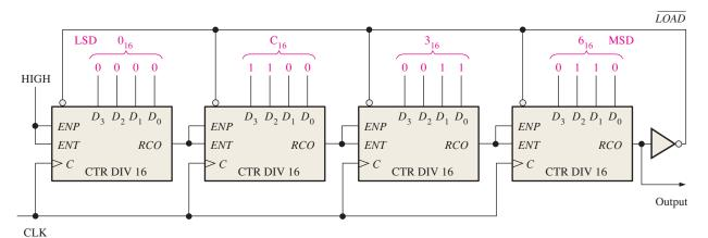
**FIGURE 9–41** A divide-by-40,000 counter using 74HC161 4-bit binary counters. Note that each of the parallel data inputs is shown in binary order (the right-most bit  $D_0$  is the LSB in each counter).
