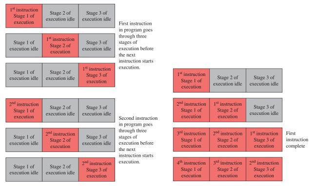
(a) Nonpipelined execution of a program showing three stages of execution
