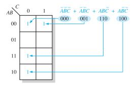
**FIGURE 4–28** Example of mapping a standard SOP expression.
