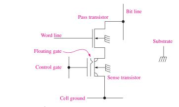
FIGURE 15-49 An E<sup>2</sup>CMOS cell.
