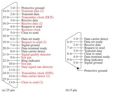
FIGURE 13–68 Standard RS-232 connectors.
