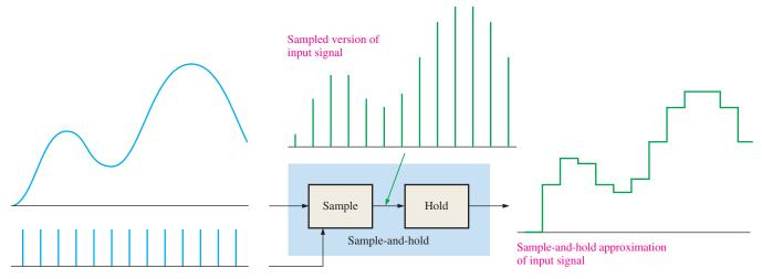
FIGURE 12–5 Illustration of a sample-and-hold operation.
