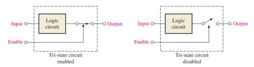
FIGURE 14-4 Logic devices with tri-state outputs.
