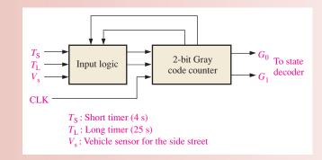
**FIGURE 7–67** Block diagram of the sequential logic.
