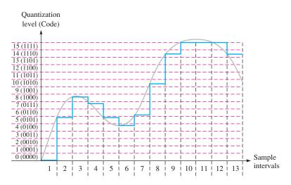
**FIGURE 12-9** Sample-and-hold output waveform with sixteen quantization levels. The original analog waveform is shown in light gray for reference.
