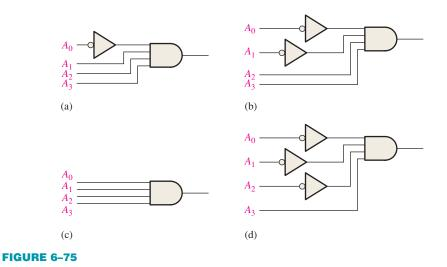
**17.** Show the decoding logic for each of the following codes if an active-HIGH (1) output is required:
