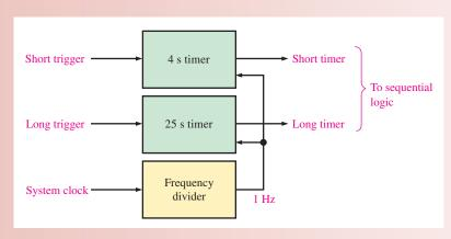
FIGURE 7–65 Block diagram of the timing circuits unit.
