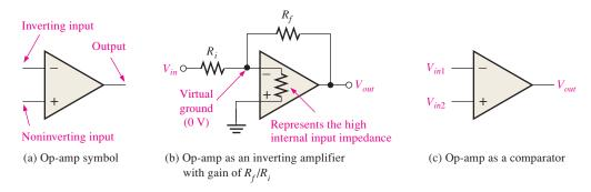
FIGURE 12-11 The operational amplifier (op-amp).
