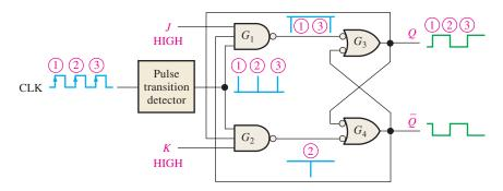
FIGURE 7-24 Transitions illustrating flip-flop operation.
