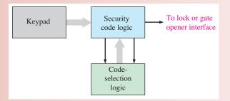
**FIGURE 8–42** Block diagram of the security system.
