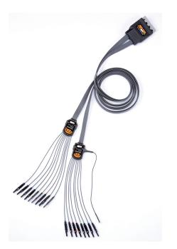
**FIGURE 1–53** A typical multichannel logic analyzer probe. Used with permission from Tektronix, Inc.
