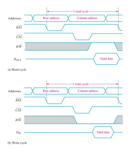
FIGURE 11-21 Timing diagrams for normal read and write cycles.
