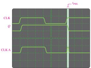
(b) Oscilloscope display showing propagation delay that creates glitch on CLK A waveform
