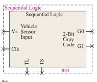
simple block symbol, as shown in Figure 10–38(b), and can be inserted as a component, as shown in Figure 10–36. A block symbol can also be created using VHDL code.
