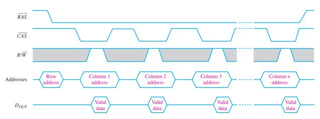
FIGURE 11–22 Fast page mode timing for a read operation.
