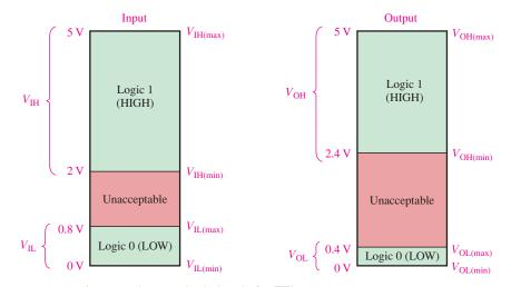
FIGURE 15–3 Input and output logic levels for TTL.
