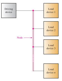
FIGURE 5-44 Illustration of a node in a logic circuit.
