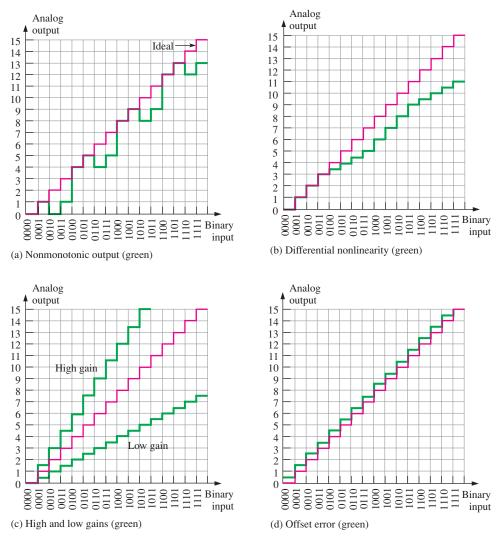
FIGURE 12–32 Illustrations of several digital-to-analog conversion errors.
