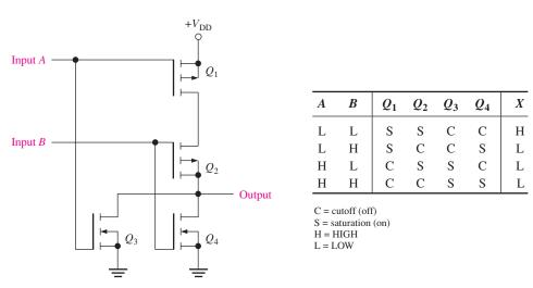
Figure 15–20 shows a CMOS NOR gate with two inputs. Notice the arrangement of the complementary pairs.
