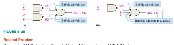
Convert the NAND circuits in Figure 5–25(a) and (b) to equivalent AND-OR logic.
