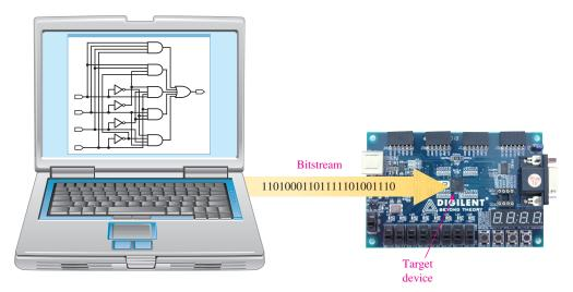
FIGURE 10-44 Downloading a design to the target device. (Photo courtesy of Digilent, Inc.)
