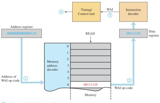
1 Address code  $(6_{10})$  is placed on address bus.
