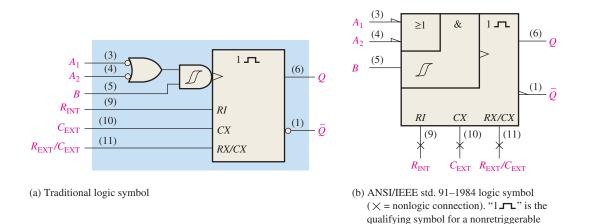
FIGURE 7-47 Logic symbols for the 74121 nonretriggerable one-shot.
