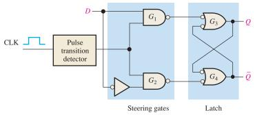
(a) A simplified logic diagram for a positive edge-triggered D flip-flop
