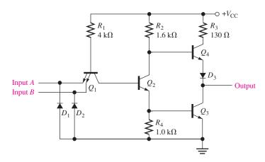
FIGURE 15–29 A TTL NAND gate circuit.
