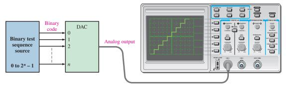
FIGURE 12-31 Basic test setup for a DAC.
