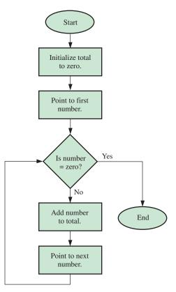
FIGURE 14–32 Flowchart for adding a list of numbers.
