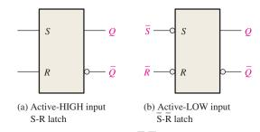
**FIGURE 7–4** Logic symbols for the S-R and  $\overline{S}$ - $\overline{R}$  latch.
