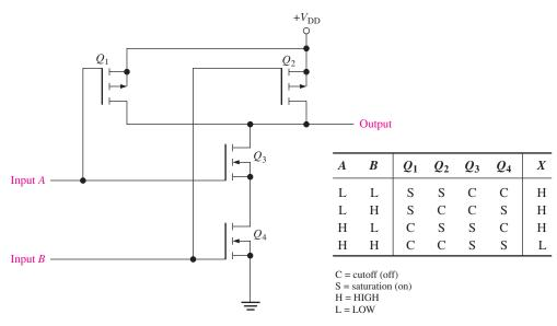
FIGURE 15–19 A CMOS NAND gate circuit.
