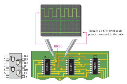
FIGURE 5-47 Shorted output in the driving device or shorted input in a load.
