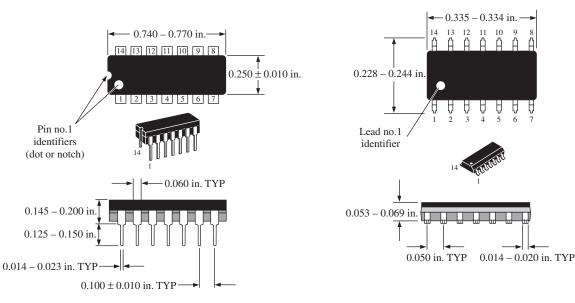
(a) 14-pin dual in-line package (DIP) for feedthrough mounting
