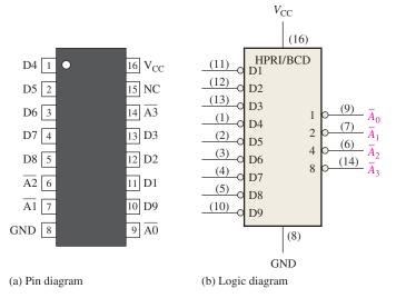
**FIGURE 6–38** The 74HC147 decimal-to-BCD encoder (HPRI means highest value input has priority.
