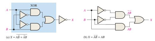
**FIGURE 5–6** Two equivalent ways of implementing the exclusive-NOR. Open files F05-06 (a) and (b) to verify the operation.
