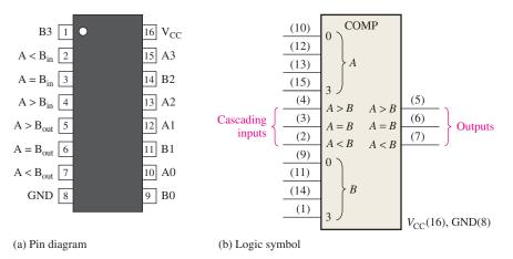
FIGURE 6-23 The 74HC85/74LS85 4-bit magnitude comparator.
