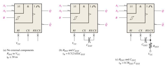
FIGURE 7-48 Three ways to set the pulse width of a 74121.
