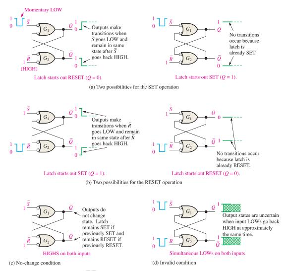
**FIGURE 7–3** The three modes of basic  $\overline{S} \cdot \overline{R}$  latch operation (SET, RESET, no-change) and the invalid condition.
