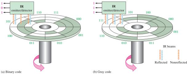
**FIGURE 2-7** A simplified illustration of how the Gray code solves the error problem in shaft position encoders. Three bits are shown to illustrate the concept, although most shaft encoders use more than 10 bits to achieve a higher resolution.
