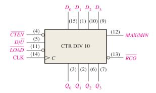
FIGURE 9-24 The 74HC190 up/down synchronous decade counter.
