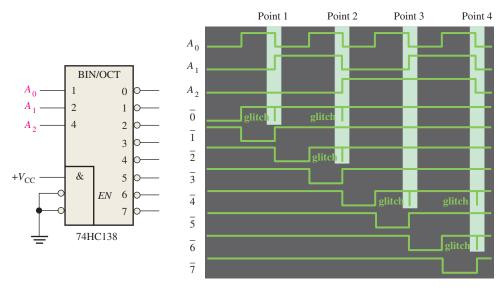
FIGURE 6-60 Decoder waveforms with output glitches.
