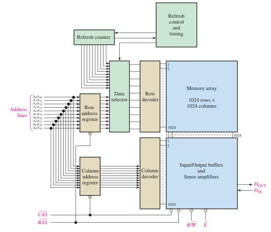
**FIGURE 11–19** Simplified block diagram of a  $1M \times 1$  DRAM.
