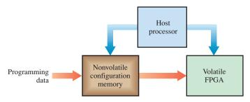
(b) Volatile FPGA with on-board memory and host processor
