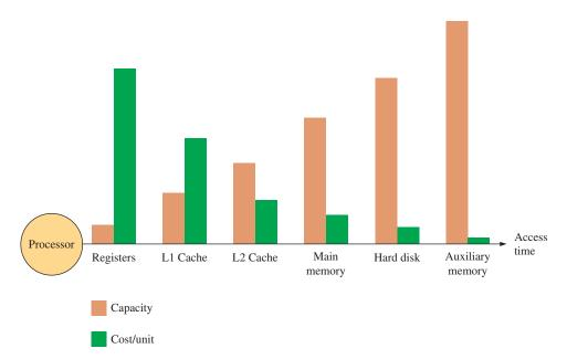
**FIGURE 11–66** Changes in memory capacity and cost per unit of data as latency (access time) increases.
