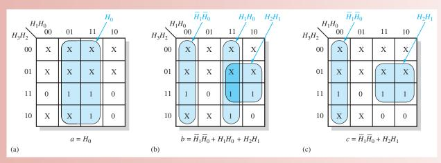
**FIGURE 4–52** Minimization of the expressions for segments *a*, *b*, and *c*.
