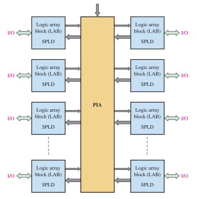
FIGURE 10-8 Basic block diagram of a generic CPLD.
