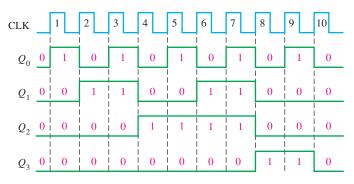
**FIGURE 9–19** Timing diagram for the BCD decade counter ( $Q_0$  is the LSB).
