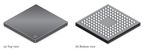
FIGURE 1-35 A typical ball-grid array (BGA) package.
