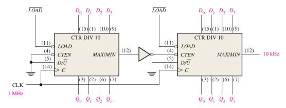
**FIGURE 9–40** A divide-by-100 counter using two 74HC190 up/down decade counters connected for the up sequence.
