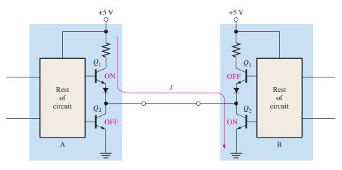
**FIGURE 15-41** Totem-pole outputs wired together. Such a connection may cause excessive current through  $Q_1$  of device A and  $Q_2$  of device B and should never be used.
