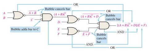
(b) Output expression can be obtained directly from the function of each gate symbol in the diagram.
