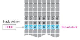
(b) The stack pointer is incremented by two and the last data word stored is copied (popped) from the stack.
