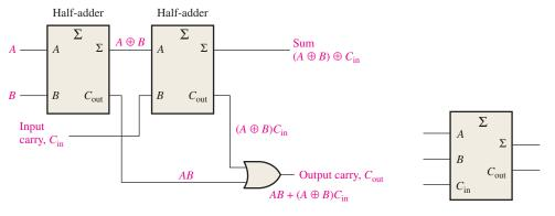
(a) Arrangement of two half-adders to form a full-adder
