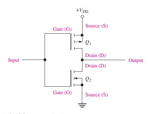
FIGURE 15–17 A CMOS inverter circuit.
