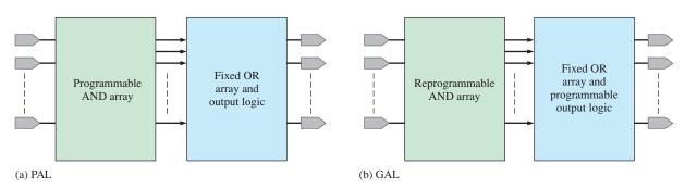
FIGURE 1-30 Block diagrams of simple programmable logic devices (SPLDs).
