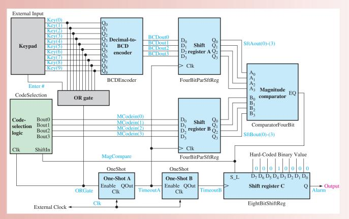
FIGURE 8-45 Security system block diagram as a programming model.
