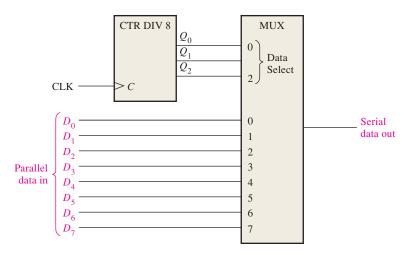
FIGURE 9–53 Parallel-to-serial data conversion logic.
