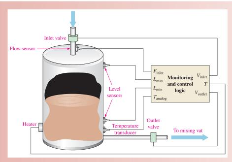
FIGURE 5–50 Tank with level and temperature sensors and controls.
