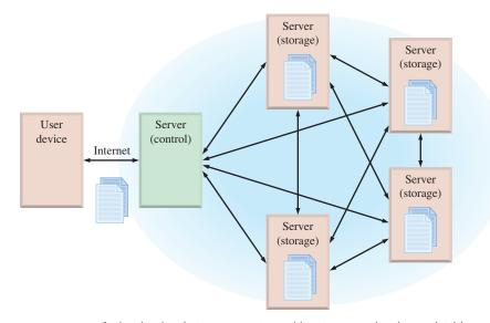
**FIGURE 11–70** A simple cloud storage system with storage redundancy. In this case, the data are stored on four different servers.
