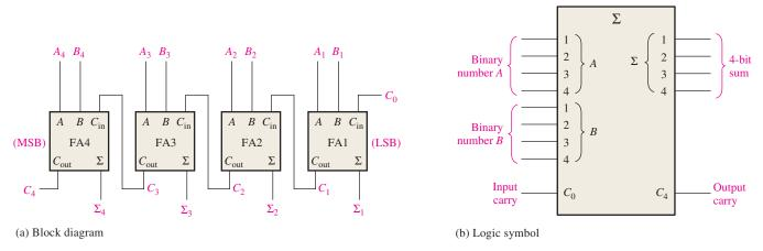
FIGURE 6-9 A 4-bit parallel adder.
