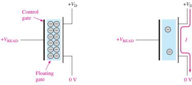
When a 0 is read, the transistor remains off because the charge on the floating gate prevents the read voltage from exceeding the turn-on threshold.
