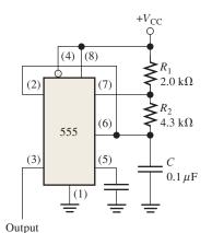
**31.** Determine the values of the external resistors for a 555 timer used as an astable multivibrator with an output frequency of 10 kHz, if the external capacitor C is 0.004  $\mu$ F and the duty cycle is to be approximately 80%.
