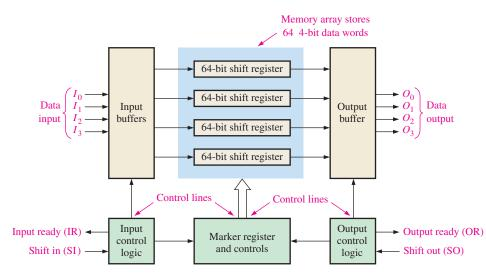
FIGURE 11–50 Block diagram of a typical FIFO serial memory.
