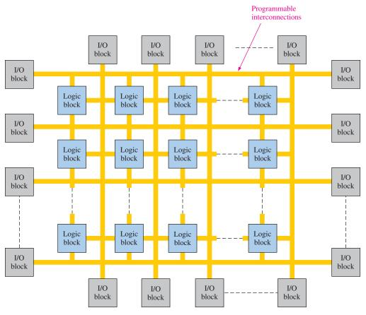
FIGURE 1-34 Basic structure of an FPGA.
