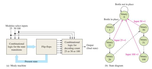
**FIGURE 9–3** A variable-modulus binary counter as an example of a Mealy state machine. The red arrows in the state diagram represent the recycle paths that depend on the input number. The black dashed lines mean the interim states are not shown for simplicity.
