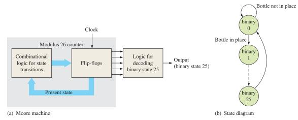
**FIGURE 9–2** A fixed-modulus binary counter as an example of a Moore state machine. The dashed line in the state diagram means the states between binary 1 and 25 are not shown for simplicity.
