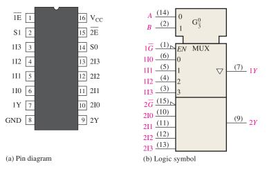
**FIGURE 6–46** The 74HC153 dual four-input data selector/multiplexer.
