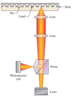
FIGURE 11-64 Basic operation of reading data from a CD-ROM.
