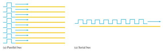
FIGURE 13–51 Comparison of parallel and serial buses.
