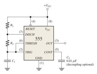
FIGURE 7-56 The 555 timer connected as an astable multivibrator (oscillator).
