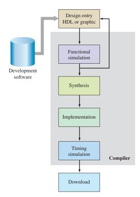
FIGURE 1-37 Basic programmable logic design flow block diagram.
