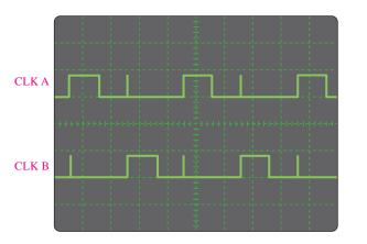
(a) Oscilloscope display of CLK A and CLK B waveforms with glitches indicated by the "spikes".
