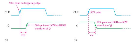
FIGURE 7-31 Propagation delays, clock to output.
