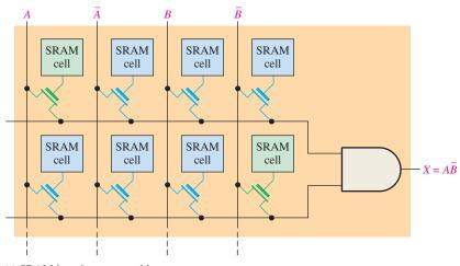
(a) SRAM-based programmable array
