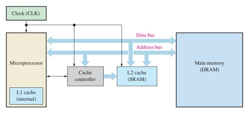
**FIGURE 11–16** Block diagram showing L1 and L2 cache memories in a computer system.
