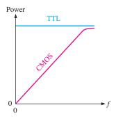
FIGURE 15–7 Power-versusfrequency curves for TTL and CMOS.
