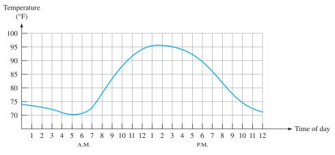
FIGURE 1-1 Graph of an analog quantity (temperature versus time).
