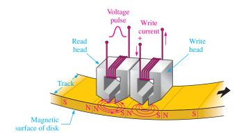
FIGURE 11-60 Simplified read/write head operation.
