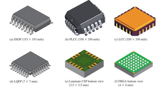
**FIGURE 1–40** Examples of SMT package configurations. Parts (e) and (f) show bottom views.
