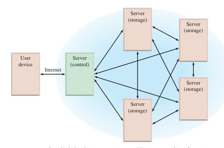
**FIGURE 11–68** A typical cloud storage system architecture consists of a master control server and several storage servers that can be accessed by a user device over the Internet.
