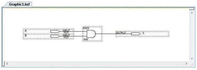
(b) Equivalent graphic (schematic) entry
