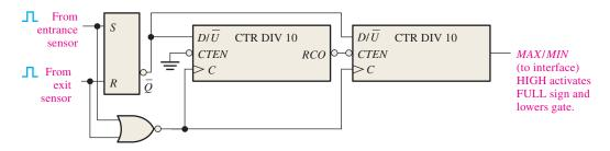
**FIGURE 9–52** Logic diagram for modulus-100 up/down counter for automobile parking control.
