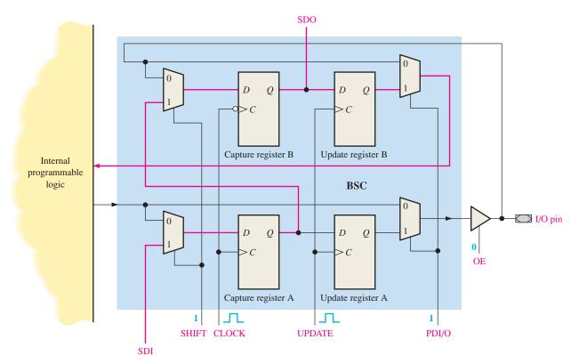
**FIGURE 10–52** Data path for transferring data from the SDI to the internal programmable logic and the SDO. There is a 1 on the SHIFT line, a 1 on the PDI/O line, and a 0 on the OE line. A pulse is applied to the CLOCK line followed by a pulse on the UPDATE line.
