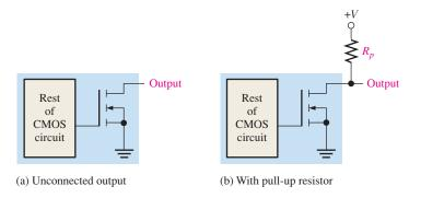
FIGURE 15-21 Open-drain CMOS gates.
