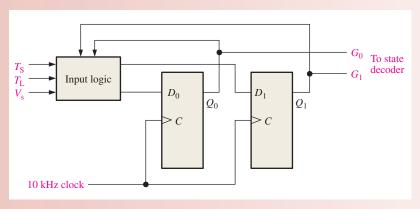
**FIGURE 7–68** Sequential logic diagram with two *D* flip-flops used to implement the 2-bit Gray code counter.
