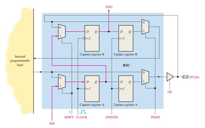
**FIGURE 10–49** Data path for serially shifting data from one BSC to the next. There is a 1 on the SHIFT input and a CLOCK pulse is applied. The red lines indicate data flow.
