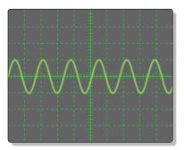
(a) Untriggered waveform display
