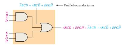
FIGURE 10-13 Basic concept of the parallel expander.
