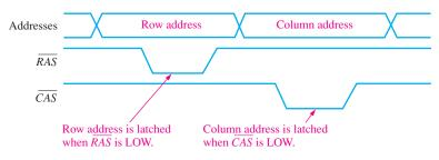
FIGURE 11-20 Basic timing for address multiplexing.
