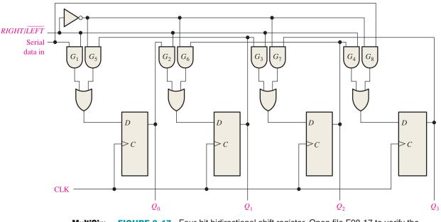
MultiSim FIGURE 8–17 Four-bit bidirectional shift register. Open file F08-17 to verify the operation.
