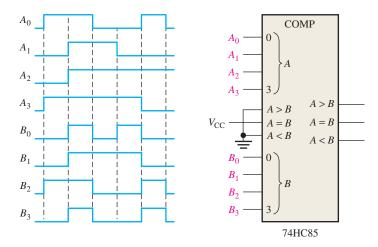
15. For each set of binary numbers, determine the output states for the comparator of Figure 6–21.
