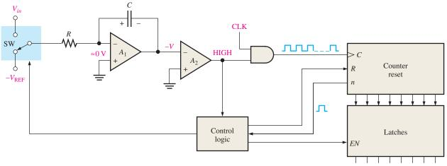
(b) End of fixed-interval when the counter sends a pulse to control logic to switch SW to the  $-V_{\text{REF}}$  input
