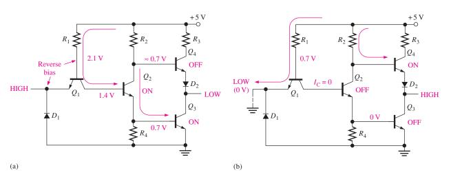
FIGURE 15–28 Operation of a TTL inverter.
