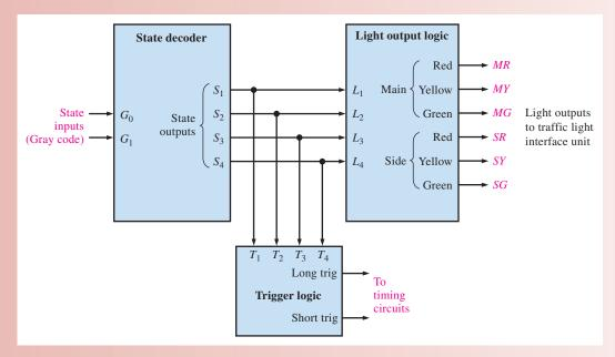
FIGURE 6-65 Block diagram of the combinational logic unit.
