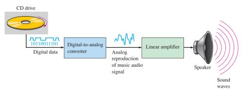
FIGURE 1-4 Basic block diagram of a CD player. Only one channel is shown.
