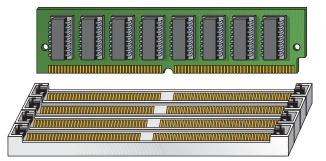
FIGURE 11-48 A memory module with connectors.
