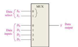
FIGURE 6-43 Logic symbol for a 1-of-4 data selector/multiplexer.
