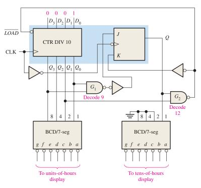
**FIGURE 9–50** Logic diagram for hours counter and decoders. Note that on the counter inputs and outputs, the right-most bit is the LSB.
