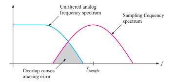
**FIGURE 12–3** A basic illustration of the condition  $f_{sample} < 2f_{a(max)}$ .
