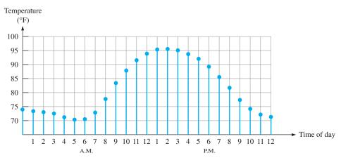
**FIGURE 1–2** Sampled-value representation (quantization) of the analog quantity in Figure 1–1. Each value represented by a dot can be digitized by representing it as a digital code that consists of a series of 1s and 0s.
