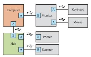
FIGURE 13-66 Example of USB applications.
