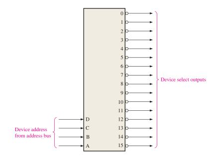
FIGURE 14-6 Address decoding for the purpose of device selection.
