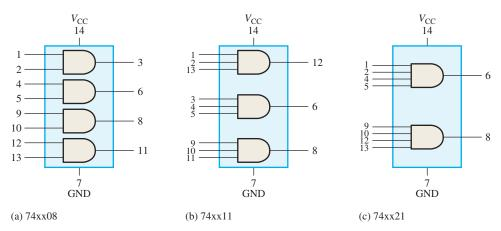
FIGURE 3-59 74 series AND gate devices with pin numbers.
