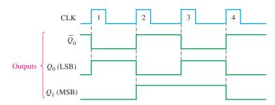
**FIGURE 9–5** Timing diagram for the counter of Figure 9–4. As in previous chapters, output waveforms are shown in green.
