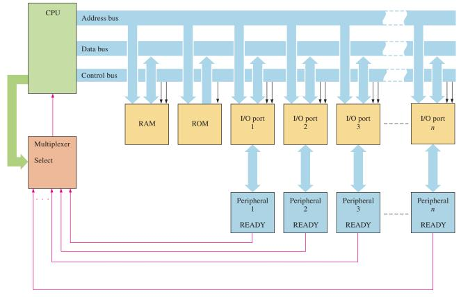
FIGURE 14–22 Basic concept of CPU polling peripheral devices.
