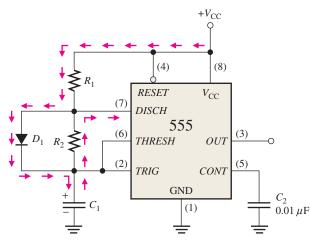
**FIGURE 7–59** The addition of diode  $D_1$  allows the duty cycle of the output to be adjusted to less than 50 percent by making  $R_1 < R_2$ .
