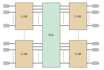
**FIGURE 1–32** General block diagram of a CPLD.
