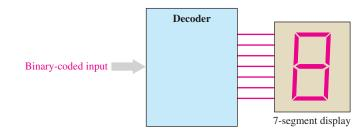
**FIGURE 1–23** A decoder used to convert a special binary code into a 7-segment decimal readout.
