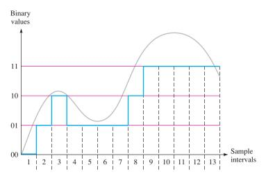
**FIGURE 12–8** The reconstructed waveform in Figure 12–7 using four quantization levels (2 bits). The original analog waveform is shown in light gray for reference.
