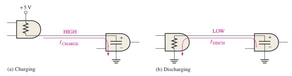
FIGURE 15-11 Capacitive loading of a CMOS gate.
