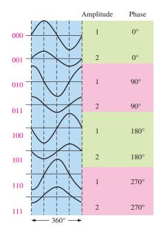
**FIGURE 13–23** Eight amplitude/phase combinations (modulation states) represent one of the eight 3-bit groups. Only one cycle of each modulation state is shown.
