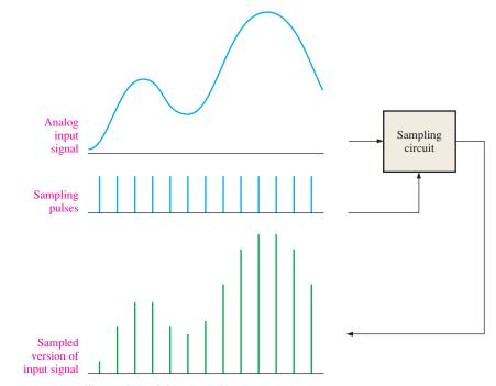
FIGURE 12-1 Illustration of the sampling process.
