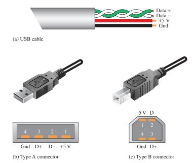
FIGURE 13-63 USB cable and connectors for USB standards through 2.0.
