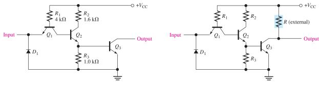
(a) Open-collector inverter circuit
