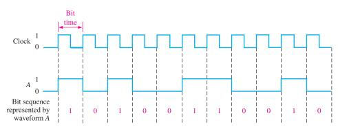
**FIGURE 1–11** Example of a clock waveform synchronized with a waveform representation of a sequence of bits.
