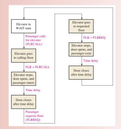
**FIGURE 9–60** One cycle of the elevator operation.
