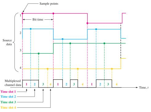
FIGURE 13-42 Illustration of TDM bit interleaving.
