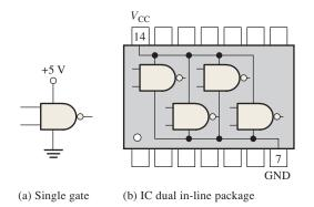
**FIGURE 15–1** Example of  $V_{CC}$  and ground connection and distribution in an IC package. Other pin connections are omitted for simplicity.
