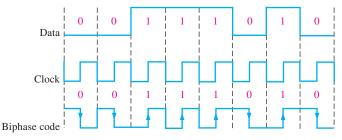
FIGURE 13–16 Example of Manchester encoded data and timing.
