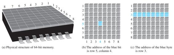
FIGURE 11-2 Examples of memory address in a 2-dimensional memory array.
