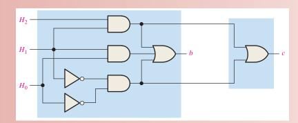
**FIGURE 4–53** Segment-*b* and segment-*c* logic circuits.
