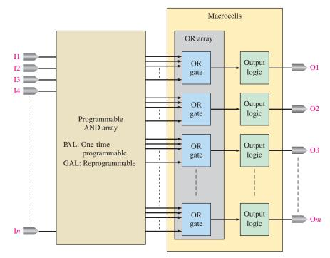
The programmable AND array outputs go to fixed OR gates that are connected to additional output logic. An OR gate combined with its associated output logic is typically called a *macrocell*. The complexity of the macrocell depends on the particular device, and in GALs it is often reprogrammable.
