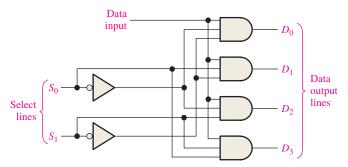
**FIGURE 6–52** A 1-line-to-4-line demultiplexer.
