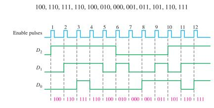
**FIGURE 12–14** Resulting digital outputs for sample-and-hold values. Output  $D_0$  is the LSB of the 3-bit binary code.
