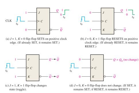
FIGURE 7–17 Operation of a positive edge-triggered J-K flip-flop.
