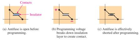
FIGURE 3–52 The programmable antifuse link.
