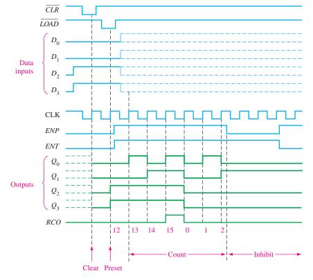
FIGURE 9–21 Timing example for a 74HC163.
