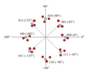
**FIGURE 13–25** Constellation map for a 3-bit PSK transmission. The phases are 0°, 45°, 90°, 135°, 180°, -45°, -90°, and -135°, as indicated.
