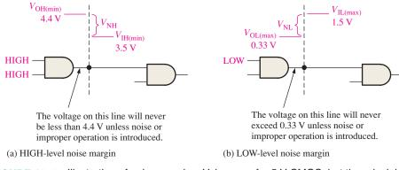
FIGURE 15-5 Illustration of noise margins. Values are for 5 V CMOS, but the principle applies to any logic family.
