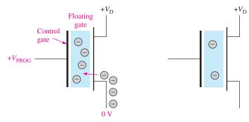
To store a 0, a sufficient positive voltage is applied to the control gate with respect to the source to add charge to the floating gate during programming.
