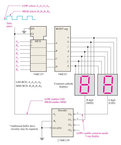
FIGURE 6-49 Simplified 7-segment display multiplexing logic.
