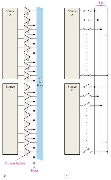
FIGURE 13-76 Tri-state buffer interface to a bus.
