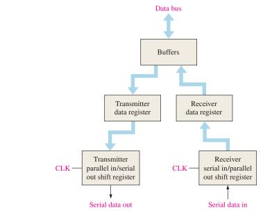
FIGURE 8–35 Basic UART block diagram.
