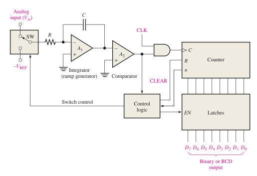
FIGURE 12-15 Basic dual-slope ADC.
