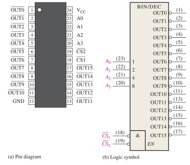
FIGURE 6–29 The 74HC154 1-of-16 decoder.
