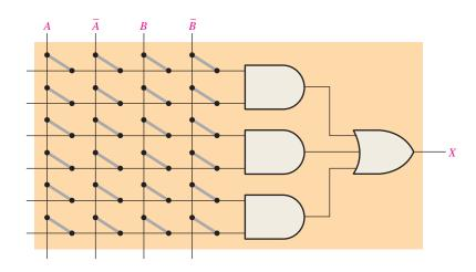
FIGURE 10-1 Basic AND/OR structure of a PAL.
