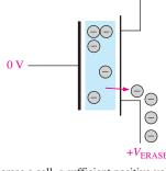
To erase a cell, a sufficient positive voltage is applied to the source with respect to the control gate to remove charge from the floating gate during the erase operation.
