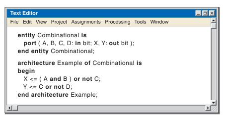
**FIGURE 5–42** A VHDL program for a combinational logic circuit after entry on a generic text editor screen that is part of a software development tool.
