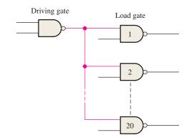
**FIGURE 3–68** The LS family NAND gate output fans out to a maximum of 20 LS family gate inputs.
