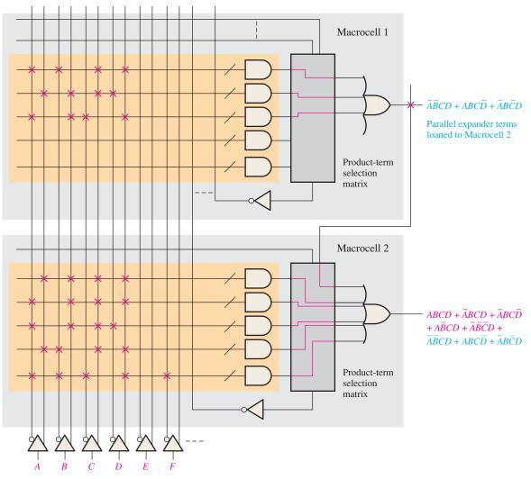
**FIGURE 10–14** Simplified illustration of using parallel expander terms from another macrocell to increase an SOP expression. The red Xs and lines represent the connections produced in the hardware by the software complier running the programmed design.
