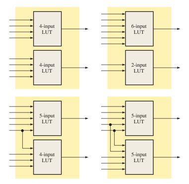
**FIGURE 10–28** Examples of possible LUT configurations in a logic module (LM) in the normal mode.
