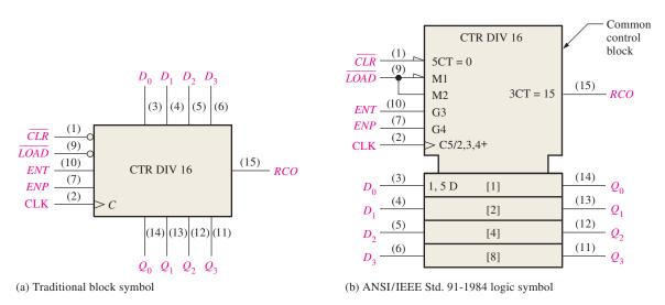
FIGURE 9–55 The 74HC163 4-bit synchronous counter.
