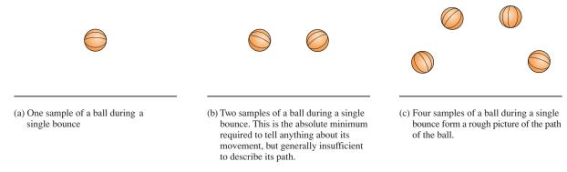
FIGURE 12–2 Bouncing ball analogy of sampling theory.
