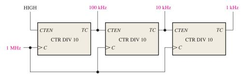
**FIGURE 9–38** Three cascaded decade counters forming a divide-by-1000 frequency divider with intermediate divide-by-10 and divide-by-100 outputs.
