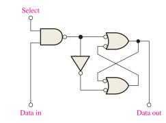
FIGURE 11-9 A typical SRAM latch memory cell.
