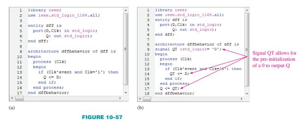
Initializing the D flip-flop output to 0 allows the Boolean expressions for D0 and D1 to resolve to a value of 1 or 0. A second simulation shows that the sequential logic portion of the traffic signal controller is now able to output a valid Gray code, as shown in Figure 10–58.
