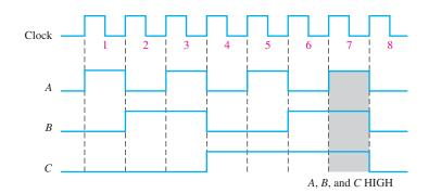
FIGURE 1-12 Example of a timing diagram.
