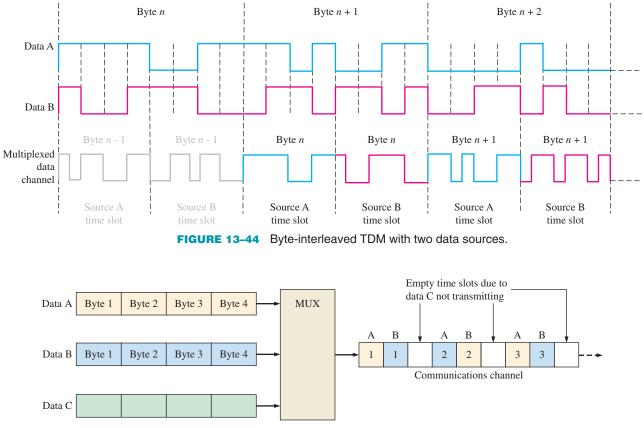
FIGURE 13-45 Example of a 3-source synchronous TDM with one data source inactive.
