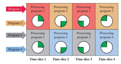
FIGURE 14–27 Multitasked multiprocessing in a multicore processor.
