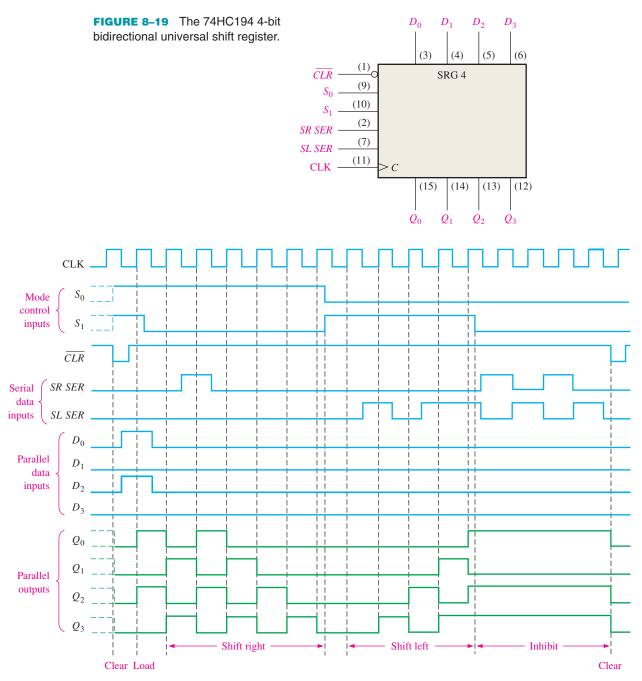
FIGURE 8–20 Sample timing diagram for a 74HC194 shift register.
