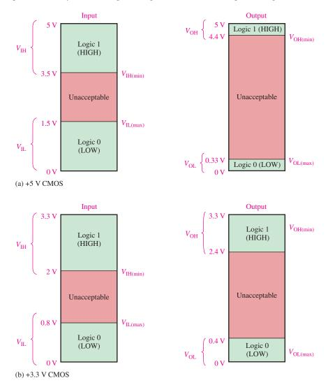
FIGURE 15-2 Input and output logic levels for CMOS.
