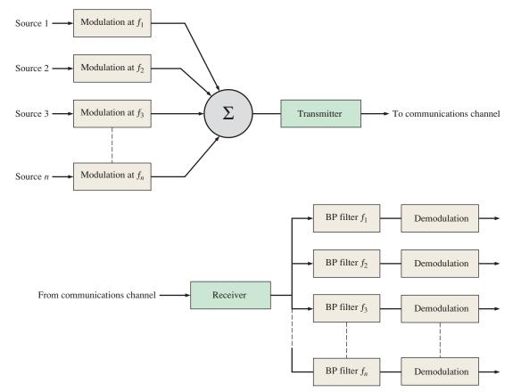
As mentioned, all sources transmit at the same time but at different frequencies. The general spectrum of a composite FDM transmission is shown in Figure 13–49. The bandwidth (BW) of each source is centered around the carrier frequency for that source and is separated from the adjacent bandwidths by the guard band.
