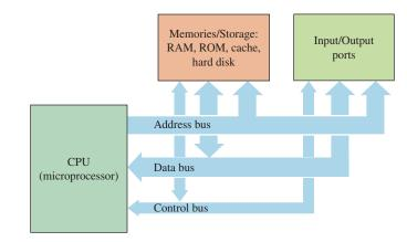
FIGURE 14-1 Basic computer block diagram.
