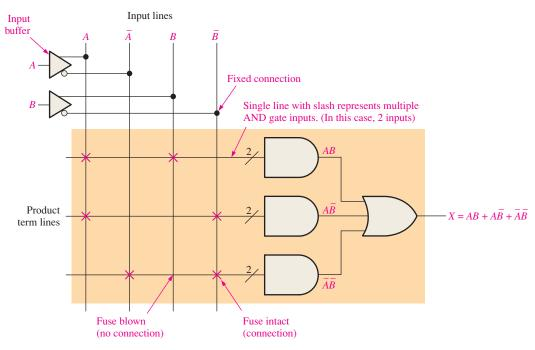
**FIGURE 10–4** A portion of a programmed PAL/GAL.
