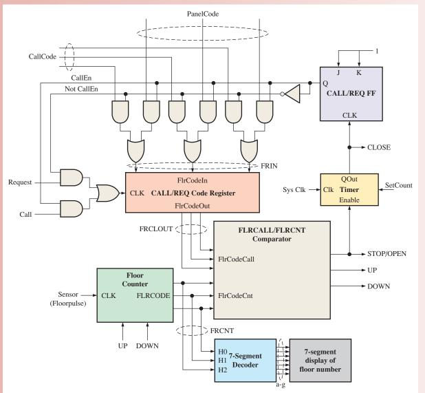
FIGURE 10-62 Programming model of the elevator controller.
