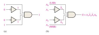
FIGURE 6-26 Decoding logic for the binary code 1001 with an active-HIGH output.
