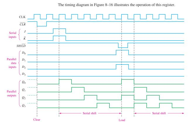
FIGURE 8–16 Sample timing diagram for a 74HC195 shift register.
