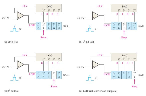
FIGURE 12–18 Illustration of the successive-approximation conversion process.
