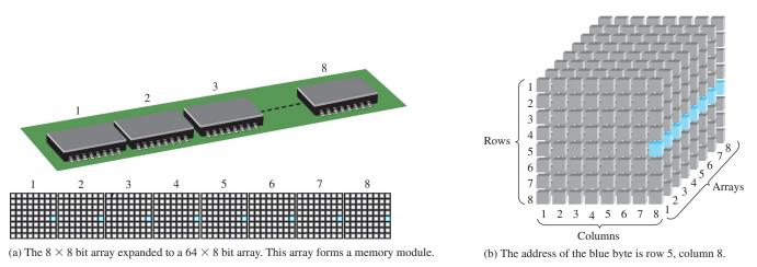
**FIGURE 11–3** Example of memory address in an expanded (multiple) array.
