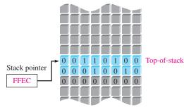
(a) The stack pointer is at FFEC before the data word is copied (popped) from the stack.
