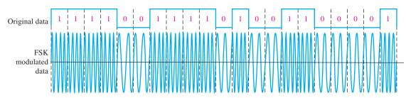
FIGURE 13–21 Illustration of frequency-shift keying (FSK).
