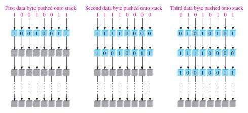
FIGURE 11-53 Simplified illustration of pushing data onto the stack.
