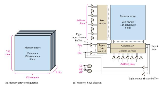
FIGURE 11–12 Basic organization of an asynchronous  $32k \times 8$  SRAM.
