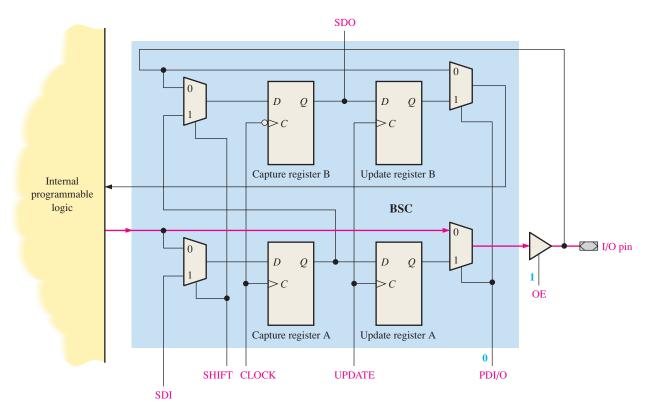
**FIGURE 10–50** Data path for transferring data from the internal programmable logic to a device output pin. There is a 0 on the PDI/O line and a 1 on the OE line.
