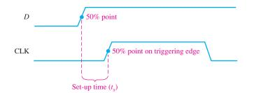
**FIGURE 7–33** Set-up time ( $t_s$ ). The logic level must be present on the *D* input for a time equal to or greater than  $t_s$  before the triggering edge of the clock pulse for reliable data entry.
