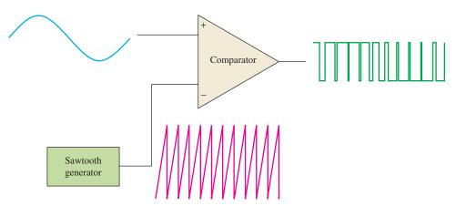
FIGURE 13-30 A basic method of pulse width modulation.
