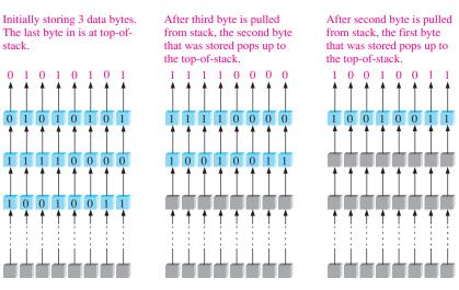
FIGURE 11–54 Simplified illustration of pulling data from the stack.
