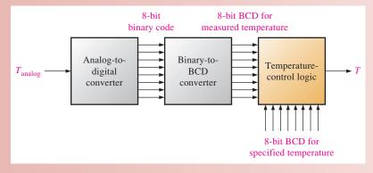
FIGURE 5–51 Block diagram for temperature control circuit.
