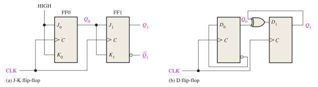
**FIGURE 9–12** 2-bit synchronous binary counters.
