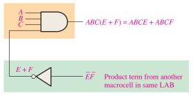
(a) A 4-input AND array gate can produce one 4-variable product term.
