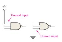
**FIGURE 15–24** Handling unused CMOS inputs.
