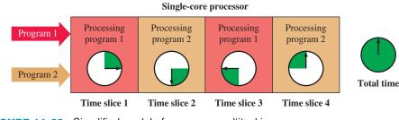
**FIGURE 14–26** Simplified model of processor multitasking.
