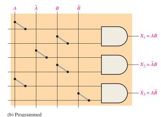
FIGURE 3-49 Concept of a programmable AND array.
