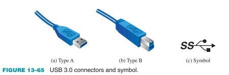
USB 3.0 is, for the most part, backward compatible with USB 2.0, but the speed is limited to the 2.0 specification. The USB 3.0 cable consists of two additional twisted pairs for data and an additional ground, for a total of nine wires. Unlike the previous versions, version 3.0 is full-duplex, meaning that data can be sent and received simultaneously. One twisted pair is for receiving data, and two additional twisted pairs are for sending high-speed data.
