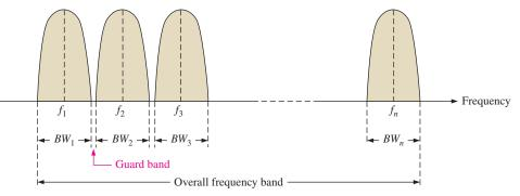
FIGURE 13–49 Frequency spectrum of an FDM transmission.
