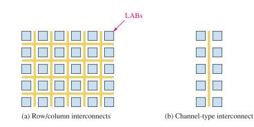
FIGURE 10-17 LUT CPLDs have row/column interconnects. Classic CPLDs have channel-type interconnects.
